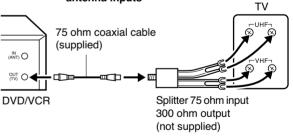
If a VHF or UHF antenna is used, set the TV/CABLE menu option to the "TV" mode.
